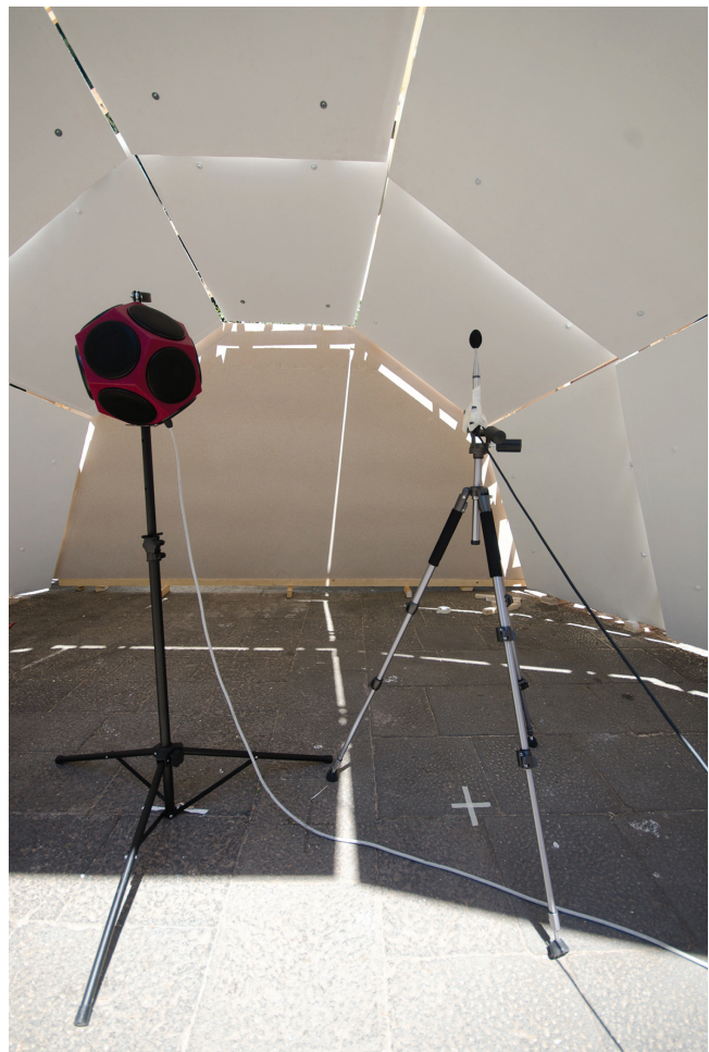
Fig. 6 A dodecahedron loudspeaker and an Ambisonic microphone used for the acoustic measurements of ReS. Ph. Sonia Ponzio.
